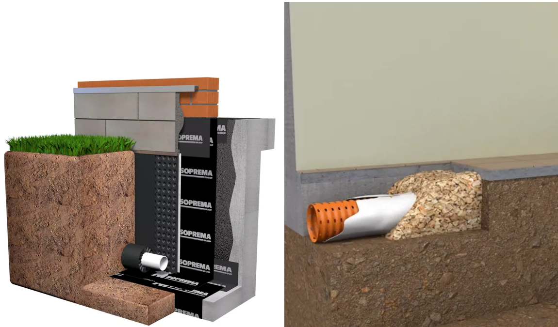
Images 12 and 13 – Waterproofing and drainage in foundations and perimeter buried walls, with construction details of exterior walls coated with ETICS solution
